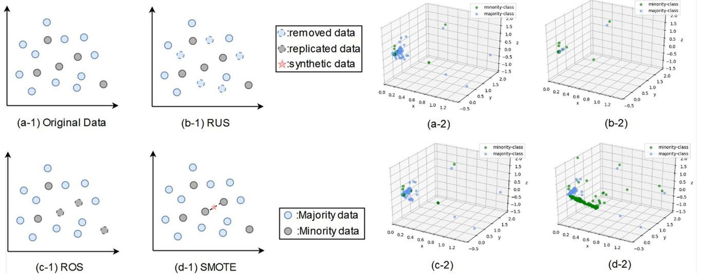
**Fig. 2.** (a-1), (b-1), (c-1), (d-1) are the illustrations of different sampling methods. The removed data are randomly selected majority samples, the replicated data are randomly selected minority samples, the synthetic data are new minority samples generated on the line linking two near neighbors in minority class. One can refer to these case studies, i.e., (a-2), (b-2), (c-2) and (d-2), for the sampling results.
