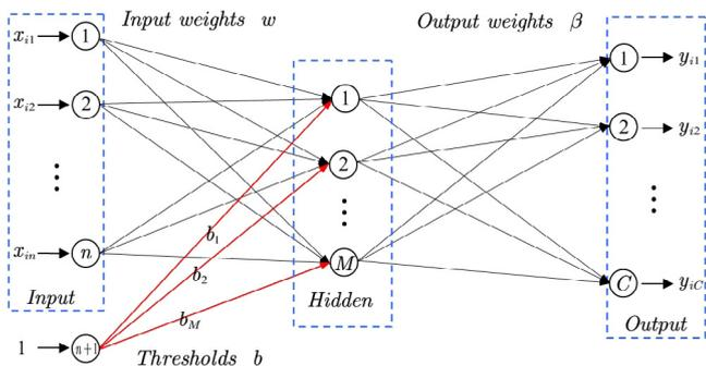
**Fig. 4.** An illustration of single hidden layer feed-forward network. This network has three layers, i.e., input, hidden and output layers with  $n + 1$ ,  $M$  and  $C$  nodes, respectively. The value of the  $(n + 1)$ th node in input layer is fixed as one, and is connected with the thresholds. The arrows indicate the direction of data propagation.
