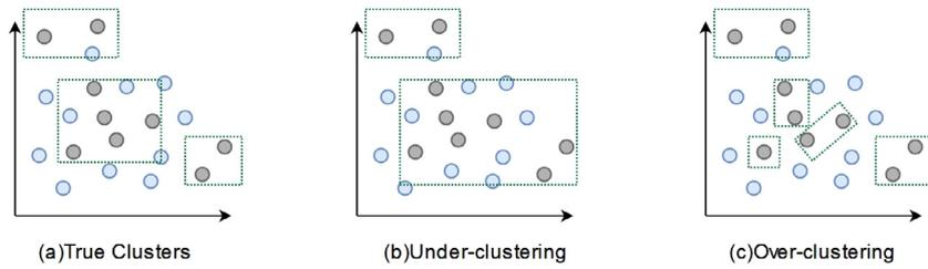
**Fig. 6.** The groups in minority class dataset. Each green frame denotes a subset in minority data. (a) shows the true but unknown division with respect to the minority class data. (b) shows a fail case with inadequate representation about minority sub-concepts. (c) shows the redundant groups in one minority sub-concept. (For interpretation of the references to color in this figure legend, the reader is referred to the web version of this article.)
