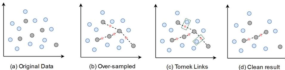
**Fig. 3.** Clean technique with Tomek Links. (a) is the original distribution of a dataset. (b) is the augmented data by linear interpolation, and the red stars are the synthetic samples. The green frames in (c) are Tomek Links which are removed for clear borderline as shown in (d). (For interpretation of the references to color in this figure legend, the reader is referred to the web version of this article.)
