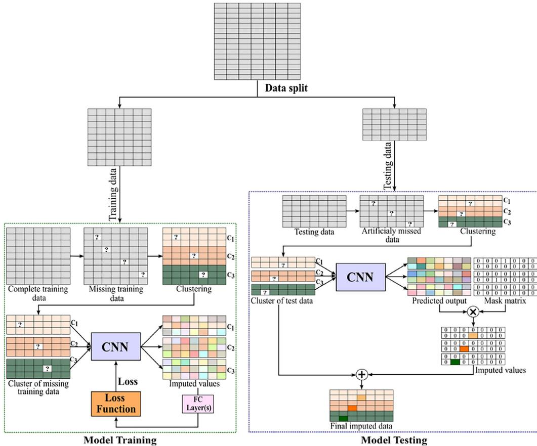
Fig. 1. Block diagram of the proposed CNNI imputation approach. One block represents model training and the other one shows the model testing.
