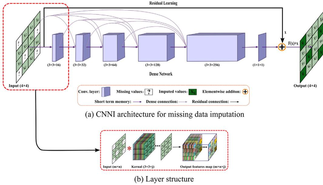
**Fig. 3.** CNNI architecture for missing data imputation is shown in Fig. 3(a). The layer structure of CNNI is shown in Fig. 3(b), which represents how each kernel (in the form of a  $3 \times 3$  matrix) convolves on the input (in the form of a  $m \times n$  matrix) and then a feature map (in the form of a  $m \times n \times j$  tensor) is obtained as an output, where the symbol  $*$  represents the convolution operation.
