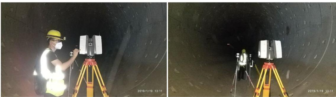
Fig. 10 Schematic diagram of independent station setup method
