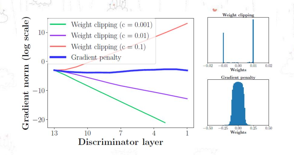
(left) Gradient norms of deep WGAN critics during training on toy datasets either explode or vanish when using weight clipping, but not when using a gradient penalty. (right)Weight clipping (top) pushes weights towards two values (the extremes of the clipping range), unlike gradient penalty (bottom).
