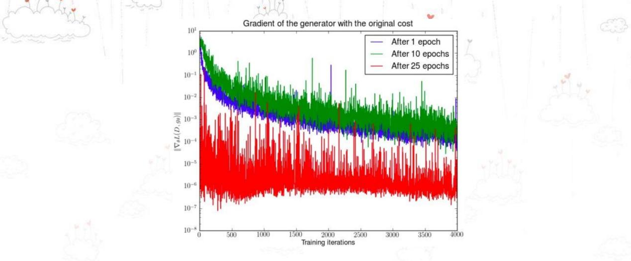
First, we trained a DCGAN for 1, 10 and 25 epochs. Then, with the generator fixed we train a discriminator from scratch and measure the gradients with the original cost function. We see the gradient norms decay quickly, in the best case 5 orders of magnitude after 4000 discriminator iterations. Note the logarithmic scale.
